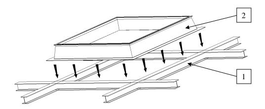
2. It is screwed on through the bottom part or heel of the crown with screws (not included) into the substructure on all sides. Screwing is carried out at intervals that match the location of the fastening screws on the skydome.
